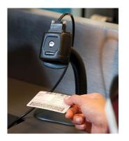
The LobbyGuard Bar Code Scanner reads the back of the driver license with 100% accuracy and can scan the visitor out of the building by scanning the bar code printed on the visitor badge.
