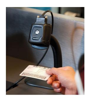
The LobbyGuard SL comes with a bar code scanner to instantly scan driver licenses with 100% accuracy. Scan the bar code on the printed visitor badge for self-service sign out.
